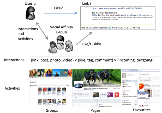
Figure 1: Overview of social affinity filtering (SAF): A social affinity group (SAG) of user u (ego) consists of a set of alternate users \{v\} (alters) who have a certain interaction or share an activity membership with u . SAF learns to classify whether user u will like item i based on the observed preferences of members of each SAG of user u toward item i .
